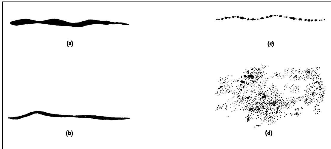
Figure 1 Indications given by Defects
