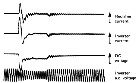
Figure 32.55 One-phase 40% fault at the inverter
