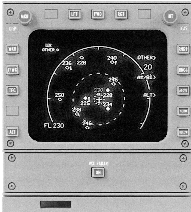
FIGURE 18.10 Joint use weather radar and traffic display.
